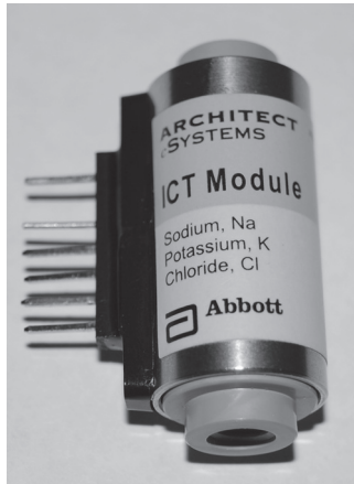
Figure 2.20 (a) Schematic of an ion selective electrode assembly; (b) Ion selective electrode module. (Adapted and reproduced with permission of Abbott Inc.)
