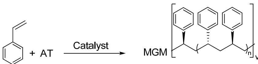
Figure 2. Catalyzed chain growth reaction. AT represents a chain transfer agent, MGM the main group metal of the chain transfer agent and v its valency.
