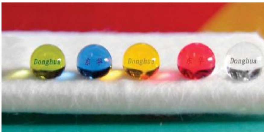
Figure 12. Several water droplets placed on the fibrous mats formed with the number ratio of syringes of 2/2 (PS/PA6) showing the superhydrophobicity.
