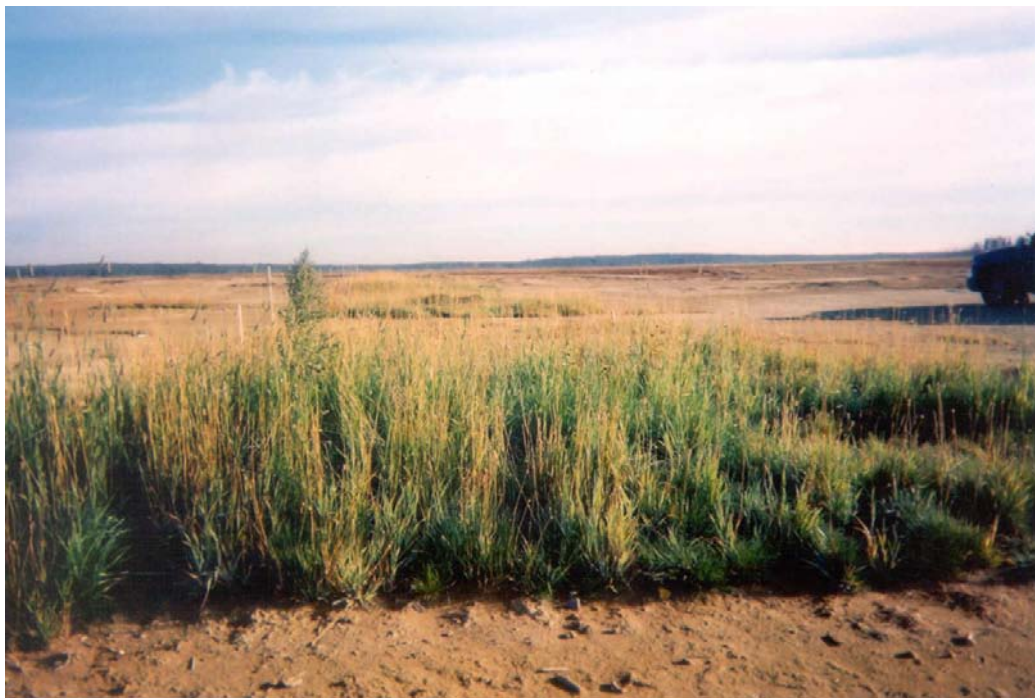
Figure 7. Organo-zeolitic treated test strip supporting grass and clover at Lynn Lake, Manitoba, Canada. This area of more than 200 hectares was covered in mine waste from sulphide mining. This site had not supported any vegetation before the test carried out in 2001. The plants have been sustained over six seasons and are still producing growth in the summer months.
