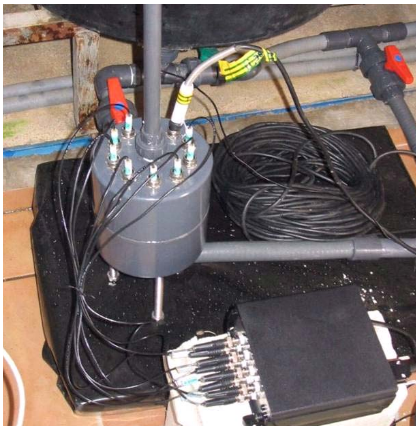
Figure 2. Installation of the electronic tongue in the on-line derivation pipe, at the IRTA site in Cabrils, with the sensor array and the multichannel potentiometer.
