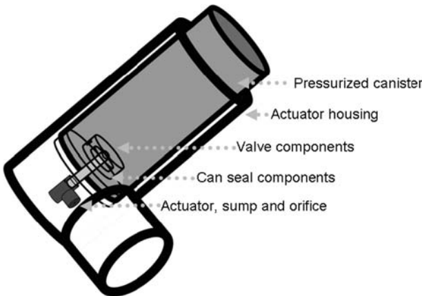
Figure 17 Schematic representation of a conventional pMDI.
