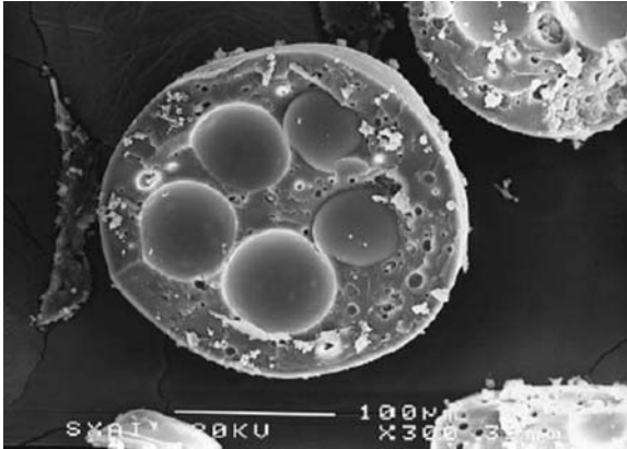
Figure 4 SEM of a cross-section of Eudragit S microparticles containing budesonide-loaded cellulose acetate butyrate cores. Source: From Ref. 21.
