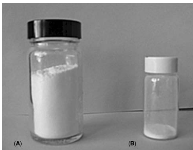
Figure 3 Powder formulations composed of: 0.75 g Itraconazole, 0.75 g Poloxamer 407, and 0.25 g Polysorbate 80. (A) Processed using the SFL technique; (B) raw unprocessed powder formulation components.
