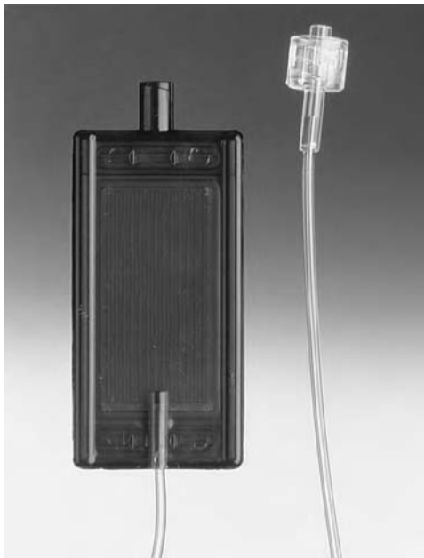
Figure 6–10 ■ Air-eliminating filter set designed for total nutrient admixture solutions. This filter has a 1.2-micron nylon membrane that provides an effective barrier for the patient from inadvertent particulate contamination, uncontrollable precipitate contamination, and entrained air. (Courtesy of Pall Corporation, Port Washington, NY.)
