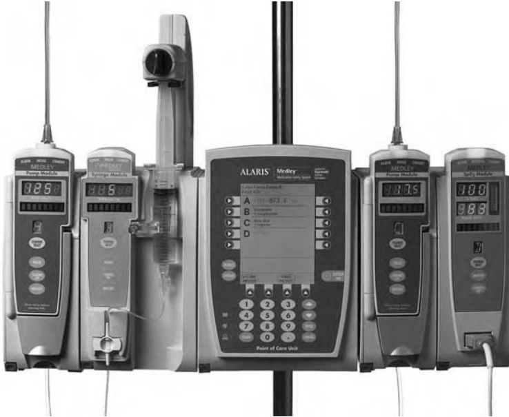
Figure 6-30 ■ Medication safety system: Modular point-of-care computer. Medley medication safety system. (Courtesy of Alaris Medical Systems, San Diego, CA.)
