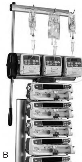
Figure 6-31 ■ Multichannel pumps. (A) Colleague CX volumetric infusion pump. (Courtesy of Baxter International Inc., Round Lake, IL.) (B) The ASENA infusion system with docking station. Volumetric pump and choice of syringe pumps. (Courtesy of Alaris Medical Systems, San Diego, CA.)
