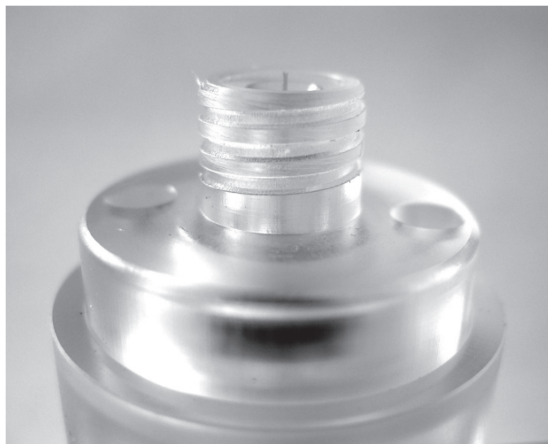
Fig. 13.7. The internal solution is applied through a fused silica capillary. The length of the capillary should be 1 mm above the inner plastic column.
