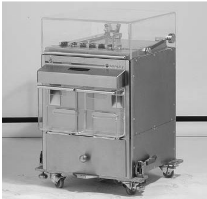
Figure 11.14 A unit for measuring tablet weight, thickness and hardness for attachment to a tablet press.
