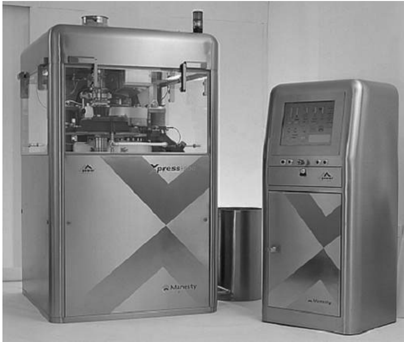
Figure 11.6 The Manesty system for the control of tablet weight.
