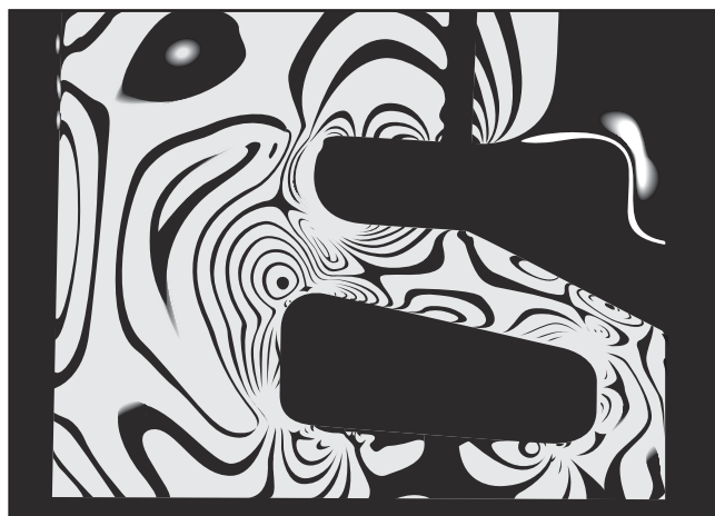
Figure 2.8 Fringes in a stressed model made from a strain-sensitive epoxy resin. (Courtesy of Sharples Photomechanics Ltd.)
