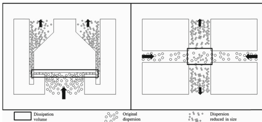
Fig. 4.17 Basic homogenization principles: piston gap ( left ) and jet-stream arrangement ( right ). In the piston gap homogenizer the macrosuspension is forced to pass through a small gap (few microns), and particle breakage is due to shear forces, cavitation, and impaction. In jet-stream homogenizers the collision of two high-velocity streams leads to particle breakage mainly by impact forces. (Adapted from R. H. Muller et al., 2006)
