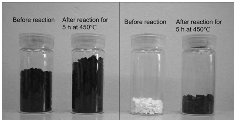
Figure 14.5 C-covered CaO (left, 160 \text{ m}^2\text{g}^{-1} , CaO: 0.1 mol) and commercial CaO (right, 7 \text{ m}^2\text{g}^{-1} , CaO: 0.1 mol) samples: C-covered CaO is bulky, fluidal, easily treated, and highly reactive. The reactivity is 10 times more than that of commercial CaO. Carbon (one of the reaction products) is deposited after the reaction on both samples.
