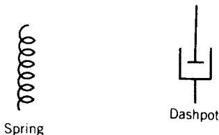
Figure 10.2 Springs and dashpots are the basic elements in modeling stress relaxation and creep phenomena.
