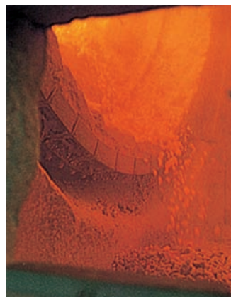
Figure 18.7 The production of CaO from \text{CaCO}_3 in a rotatory kiln.
