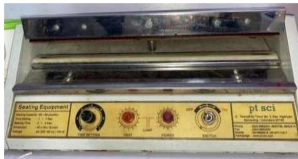
**Gambar 26.** Mesin Sealing Bungkus Puyer
